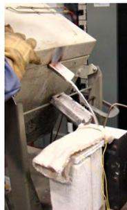
Figure 2. Pouring of casting type C.
